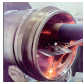
Cylinder liner repair
