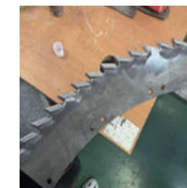
Crushing machine knife cladding
