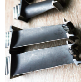
Z-notch repair of low pressure turbine blade
