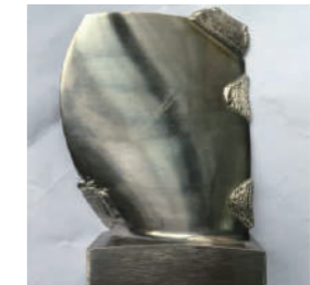
Blade notch repair
