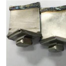
Compressor blade repair
