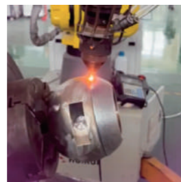
Ball valve cladding
