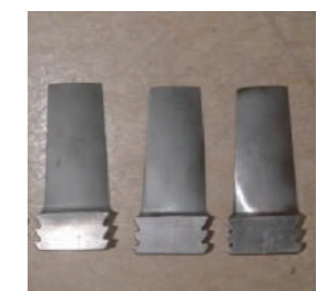
Steam turbine blade repair
