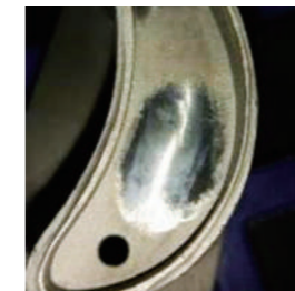
Gas turbine blade tip filling
