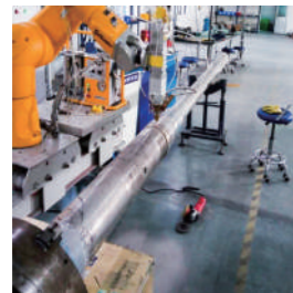
Axle wear repair
