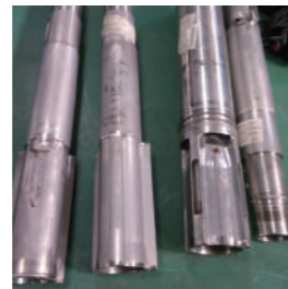
IPTA drilling tool transfer end face repair
