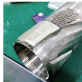
Centralizer wear repair
