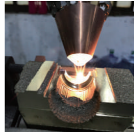
Glass mold repair
