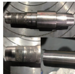
Pump shaft repair
